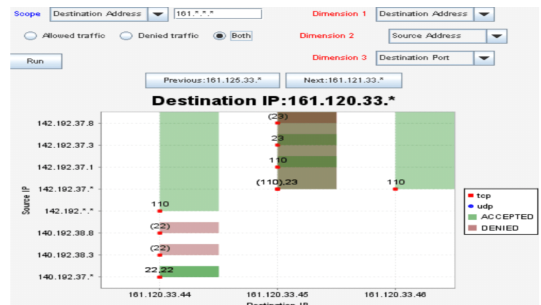
Fig. 2. Example of ACL Visualization from PolicyVis[4]
